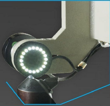
CAMERA WITH TELE CENTRIC LIGHT SOURCE AND INCIDENT LIGHT
